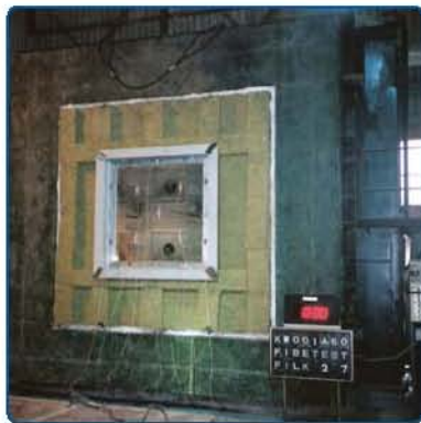
1 Ready for fire test (0min)
