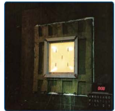
3 The pressure glass toward the furnace cracked (8 min)
